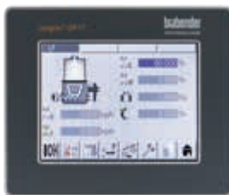
Touch screen operator interface for a single gravimetric feeder
