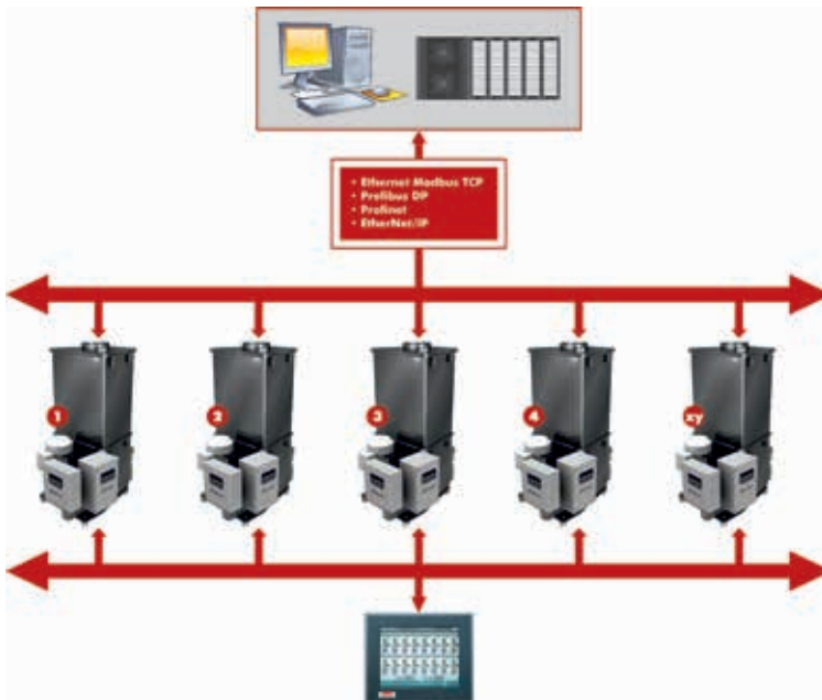
Multiple feeder control solution for gravimetric feeders with feeder mounted control modules for direct connection to a host/PLC system (optionally available with control cabinet mounted control modules)
