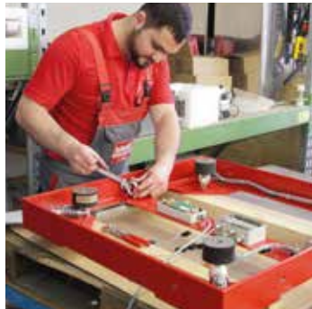
Modification of a weighing platform
