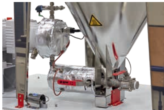
Electric trace heating on a liquid feeder
