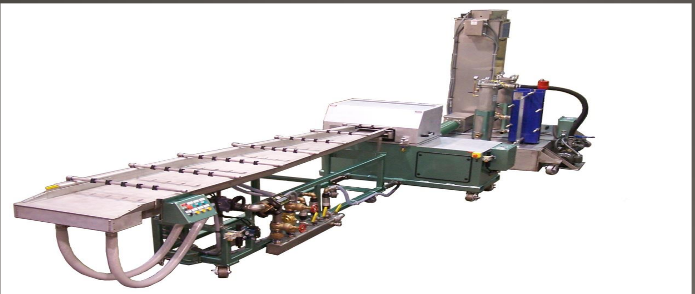
WET CUT SYSTEM WITH CENTRIFUGAL DRYER
