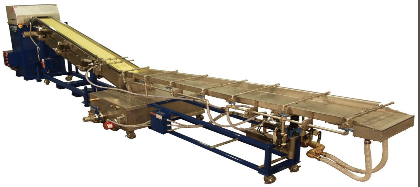
DRY CUT SYSTEM WITH WATER SLIDE AND BELT DRYER
